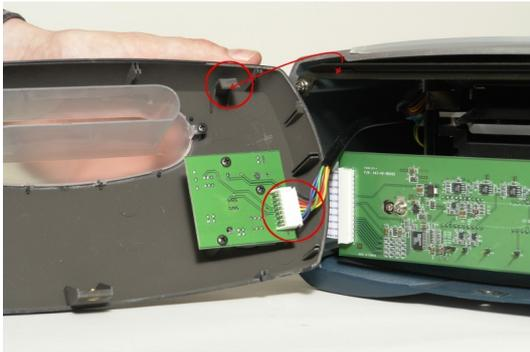
To finish the assembly fasten the front cover with the central screw on the bottom of the scanner..
