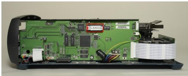
Carefully raise the chip by placing an appropriate tool between the chip and the chip holder.
