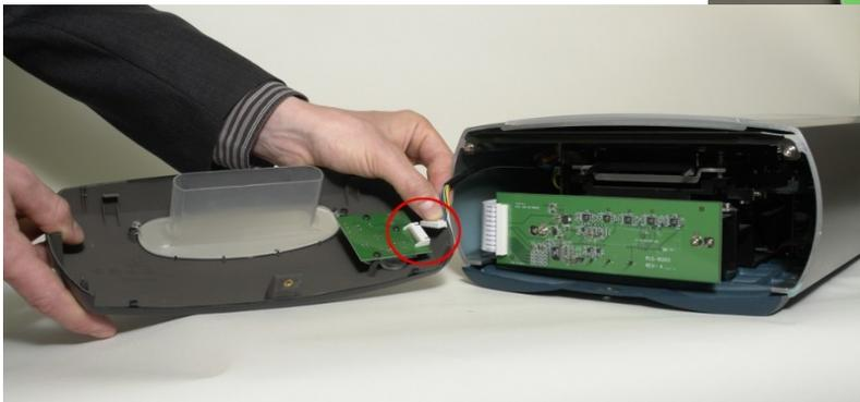
Turn the device back on its rear and remove the six side-screws holding the main cover.
