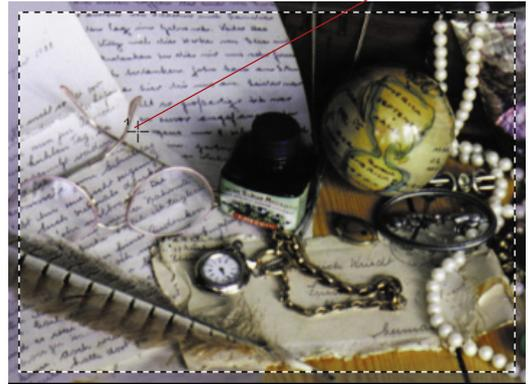
The densitometer reading before might be C27 / M25 / Y18. Now click onto the desired spot in the prescan and you will see how the CMY colours become the averaged value of C23 / M23 / Y22 – the colour tint has become neutral.
