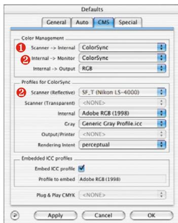
Select the scanner profiles ③ (reflective/transparency) of your scanner in section “Profiles for ColorSync” and under Output/Printer your printer profile. Select the profile of the internal system colour space under “Internal”. *SilverFast* assumes your image application supports complete colour management . Please check for this feature in the manual of your software manufacturer.
