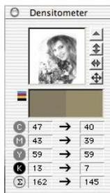
Activate the permanent softproof function and choose (e.g.) black, “K” (C, M, and Y are to be deactivated). In the prescan window, the image will now be displayed in accordance with the pre-selected separation profile.
