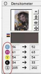
If the permanent softproof function is activated, the respective colour can be displayed in the prescan window when clicking on C, M, Y or K buttons of the densitometer.
