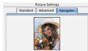
The current view can be changed by dragging the red frames (3rd illustration left), or by clicking the mouse (4th illustration left). The large preview window changes accordingly.
