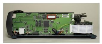
Carefully raise the chip by placing an appropriate tool between the chip and the chip holder.
