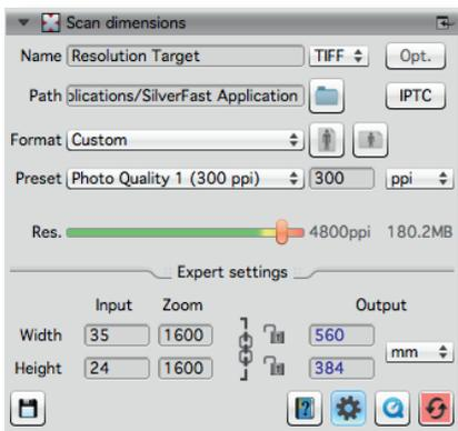
If the slider is pushed to the far right to the highest value, an **interpolated resolution** is selected, which is not suitable for scanning the Resolution Target.
