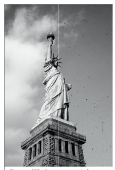
The new SRDx feature automatically removes dust and scratch artifacts from film and photographic prints. The left half of the image shows the result.
