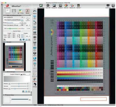
During the fully automatic profiling process, SilverFast 8 zooms in to the target. As a result, the many color measuring fields are easy to identify. All of the target data is read via barcode.
