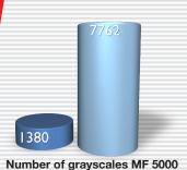
SilverFast Multi-Exposure records an original's maximum Dynamic Range by performing a double scan with a longer exposure time of the second scan. This procedure captures the highlights of the image in the first pass, and the details in the shadows during the second pass. Afterwards an algorithm calculates the final scan, which now contains all details from both scans. (LaserSoft Imaging Patent with Auto-Alignment, Patent-Nr.: EP 1744278).
